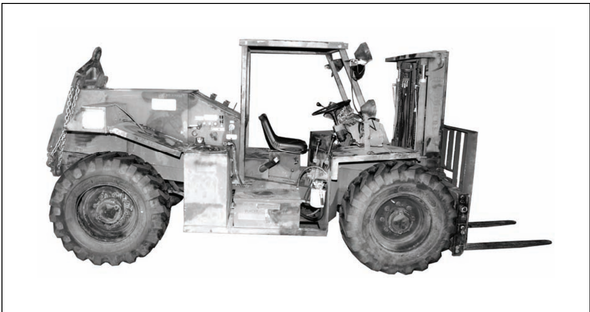
Figure 3-1. M-271, 4,000-Pound Capacity Forklift Truck with Foam Filled Tires
