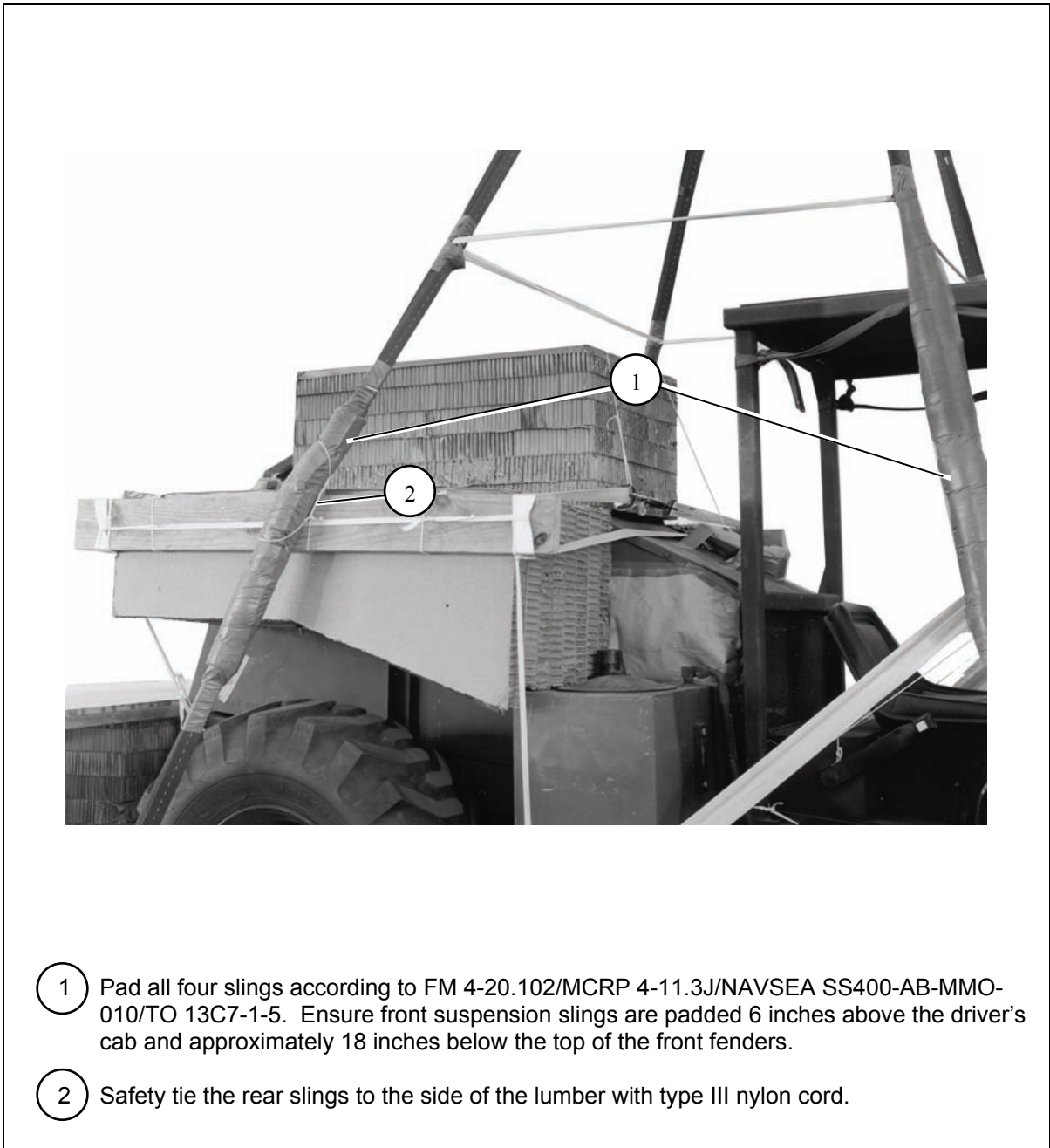
Figure 2-37. Rear Suspension Sling Safety Tied and Padded
